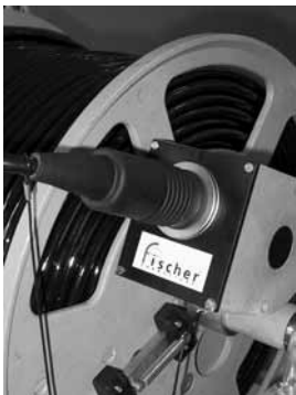
Picture 4: Plug connection on motor-driven cable drum
